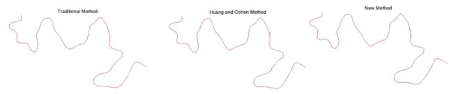
The original curve is in black. The approximated curves are in red. The new algorithm generates the least noticeable approximation errors.
