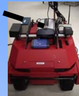
A reference station knows its exact location and broadcasts a correction message.
