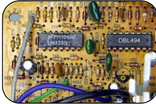
Figure 1 – A close-up of the power supply board. The LM339 and DBL494 chips can be seen, as well as the PowerGood wire (gray) and the PS-ON wire (green).
