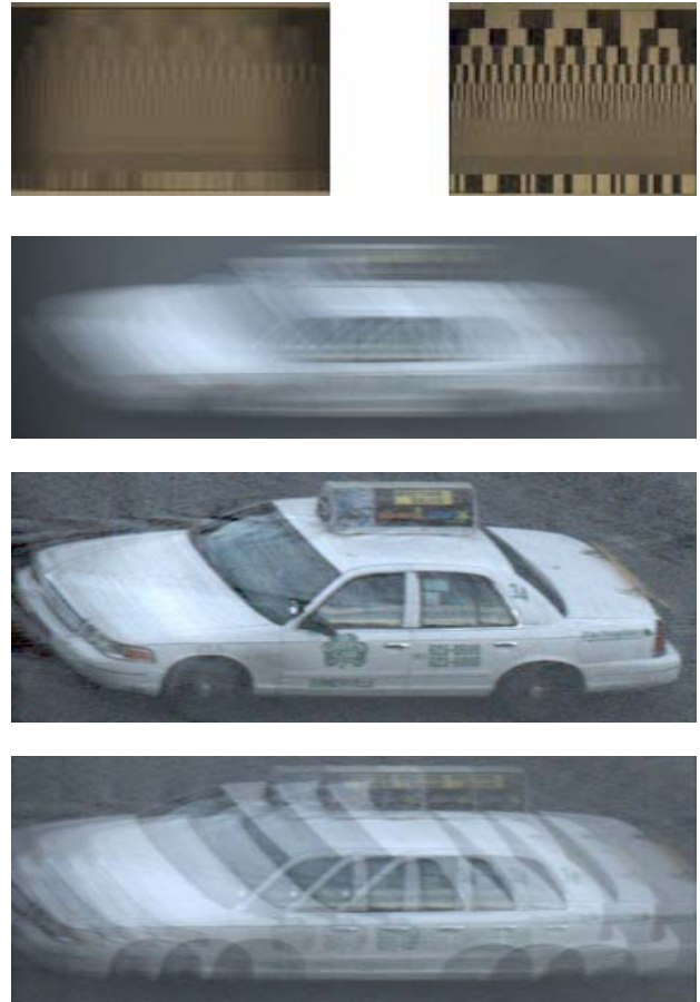
Figure 1. Blurred Frequency Grating; Restored Frequency Grating; Coded Exposure Taxi; Deblurred Taxi; Taxi modified with Ghost Blur filter.
