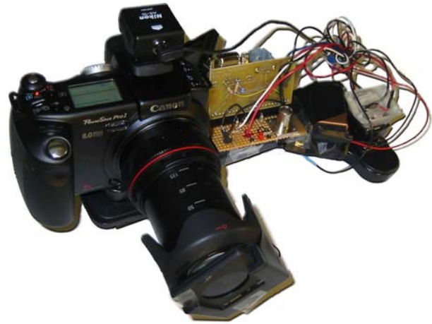
Figure 2. Digital SLR fitted with LCD Shutter.
