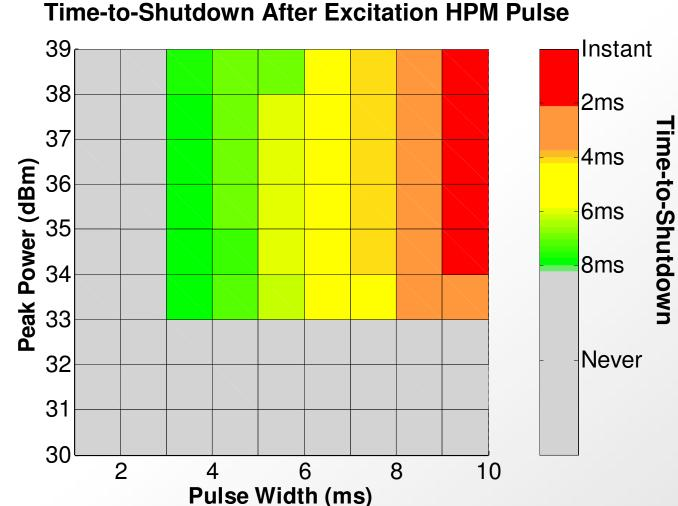
• The time-to-shutdown after pulse excitation is not linearly related to pulse width and peak power -
