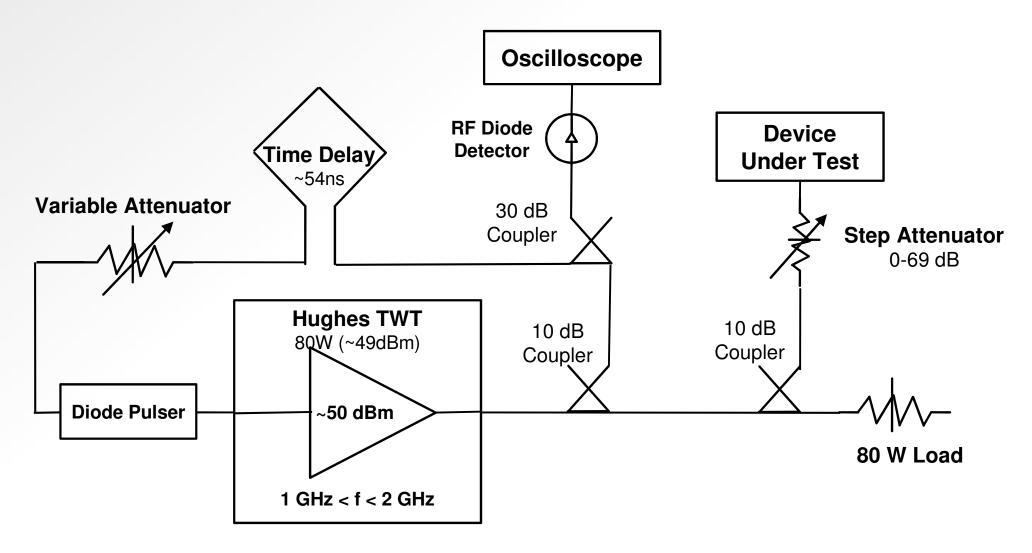
• HPM pulses of varying pulse width and power were directly injected into a power supply while monitoring DC output voltages.
