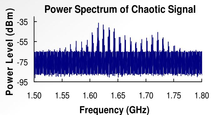
The chaotic signal had a center frequency of 1.65 GHz and a 200 MHz bandwidth, which is 4 times the bandwidth needed for 'wideband' designation.
