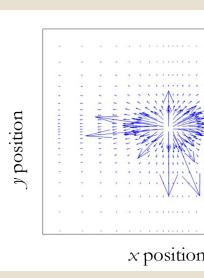
The Poisson equation is solved to obtain the electrostatic potential, capacitance, and electric field of sensor devices:
