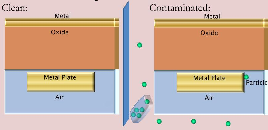
When a particle attaches to the metal plate, it is detected by measuring the capacitance change across the oxide.
