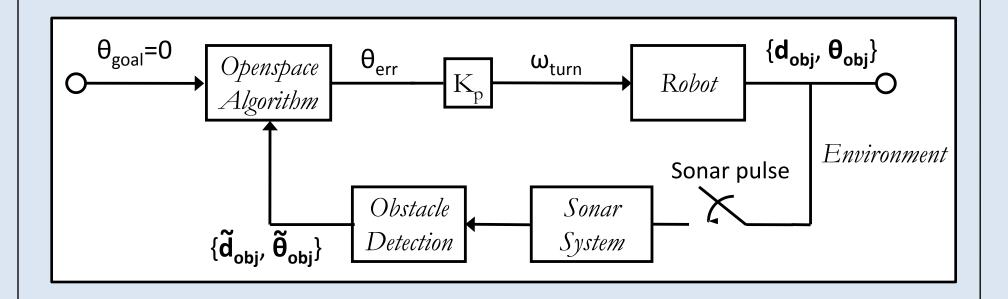
This figure details the flow of data in the real-time Once the Openspace evaluation function system. the winner-take-all angle, a calculates proportional controller adjusts the robot's movement accordingly. Then the sonar system and obstacle detection code reevaluate the environment to provide feedback.
