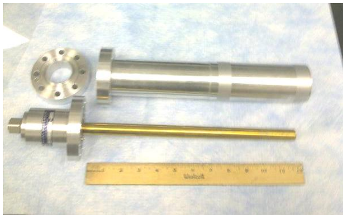
Fig 1. Cylindrical capacitor used for measurements. The inner cylindrical conductor is made of brass and has radius R1 = 16.87 mm. The outer cylindrical shell is made of aluminum and has radius R2 = 38.79 mm. Both have length l = 435 mm.
