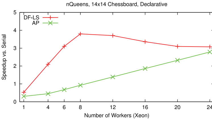
Fig. 5. Performance scaling of schedulers on Xeon (nQueens).
