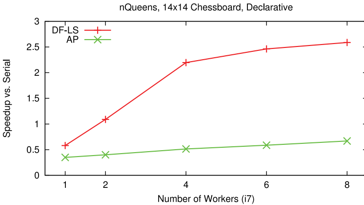
Fig. 4. Performance scaling of schedulers on i7 (nQueens).
