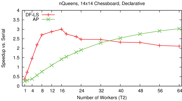
Fig. 6. Performance scaling of schedulers on T2 (nQueens).
