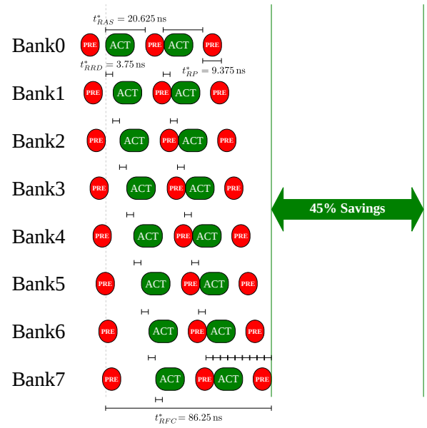
Figure 7: Example for ORGR with 2Gbit x16 DDR3 Device with r = 2 and B = 8
