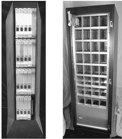
Figure 2: 16-node machine and 128-node chassis.
